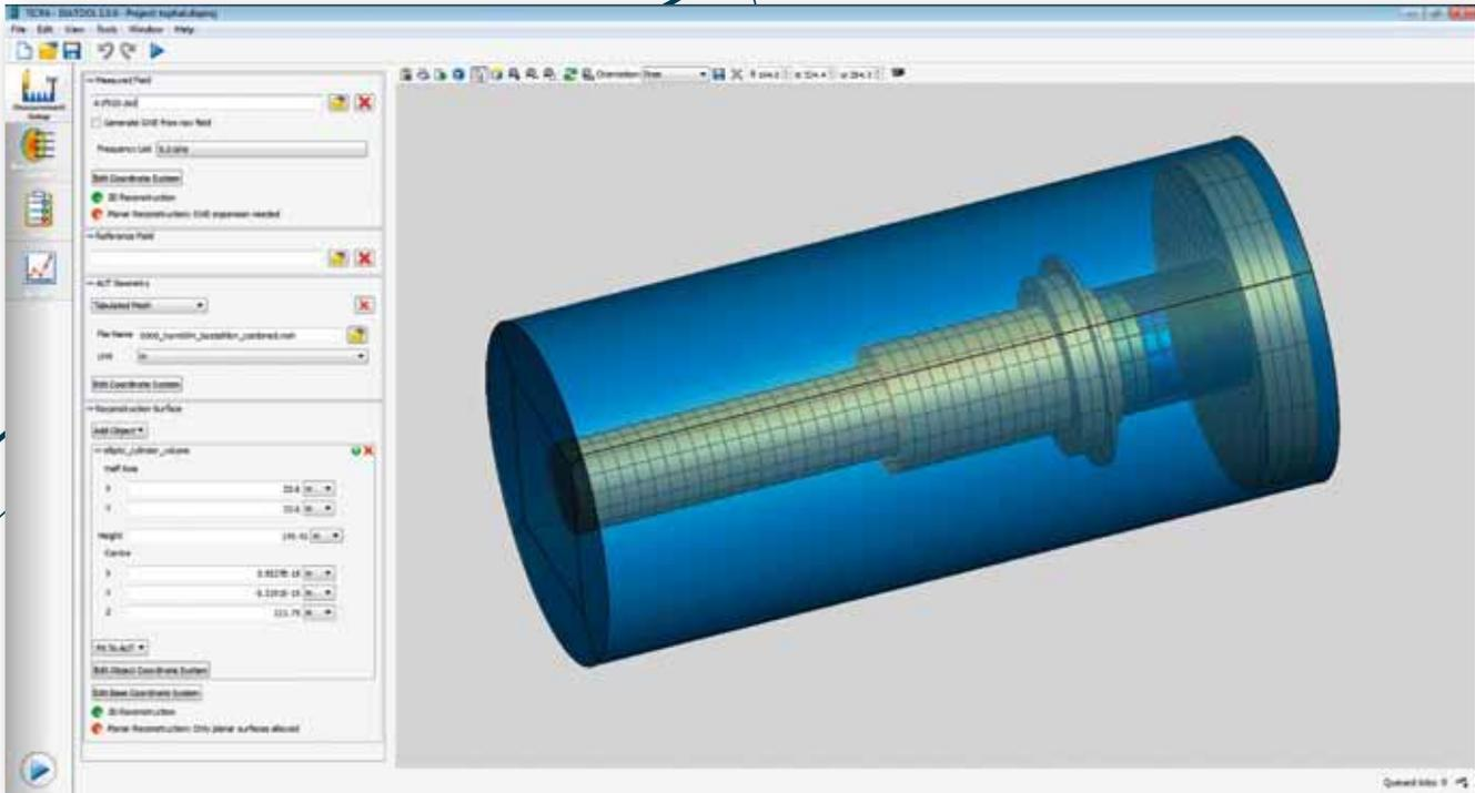
The DIATOOL GUI – Measurement Setup editor: the AUT is imported as a meshed geometry and the reconstruction surface is auto-defined as a cylinder enclosing the AUT.
