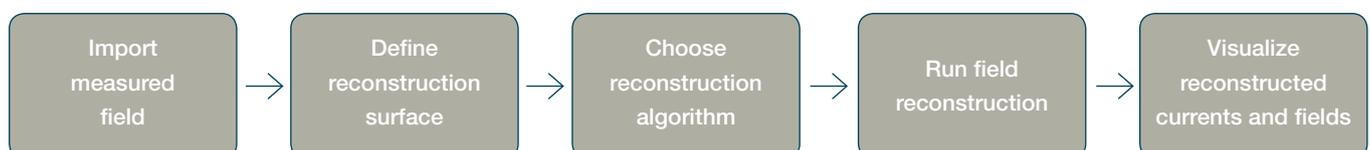
A typical field reconstruction flow with DIATOOL: in a few steps the reconstructed field is obtained.
