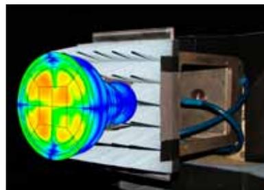
Application of the 3D reconstruction: the cross-polar component of the radiated electric field is reconstructed on a closed surface conformal to the AUT. The figure shows an unexpected asymmetry which is due to an error in the horn feeding network and which causes a high cross-polar component in the measured pattern.
