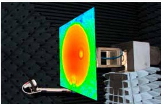
Application of the planar reconstruction: the co-polar component of the radiated electric field is reconstructed on a plane in the measurement coordinate system. A bump on the reflector surface is clearly visible. The bump caused numerous ripples in the side lobes of the measured far-field pattern, while the main lobe did not show any anomaly.
