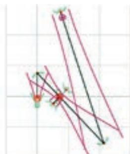
QUASt Frame drawing of Band 7 of the front end of the ALMA telescope: one of the feeds, mirrors M1 and M2 and polarization grid.
