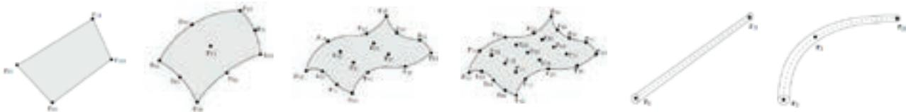
Using higher-order basis functions and curved surface patches reduces computation time and memory requirements significantly.
