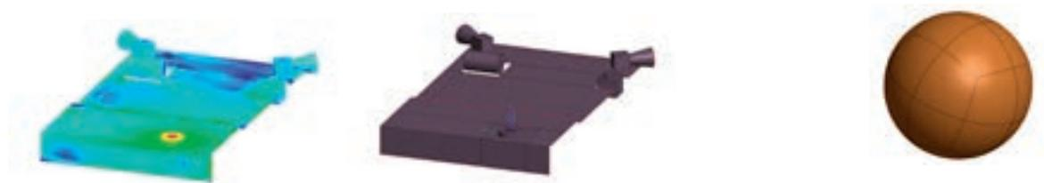
Full-wave analysis of the Exomars UHF antenna with the MoM add-on. The potential scattering in the scientific instruments on board is considered, including a major part of the satellite body.
