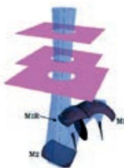
QUASt OpenGL plot of Band 7 of the front end of the ALMA telescope: feeds with mirrors M1 M1R M2, polarization grid and cryostat windows.
