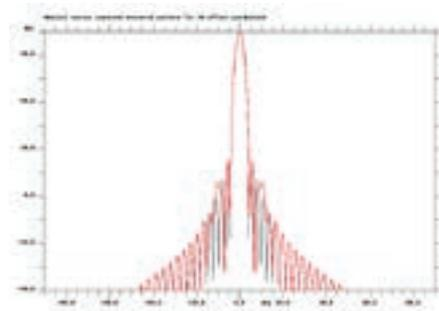
Coupling analysis of an antenna in a compact test range.
