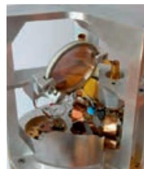
Band 7 cold optics of the front end of the ALMA telescope: mirrors M1 and M1R at the top partly hidden, circular polarization grid in the middle and mirror M2R at the bottom (IRAM, France).
