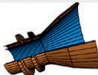
A simple conical horn section is defined by the input and output radii and the section length. In this example the horn is parameterized in terms of the flare angle, enabling optimization of, for example, the aperture radius whilst keeping the angle constant.
