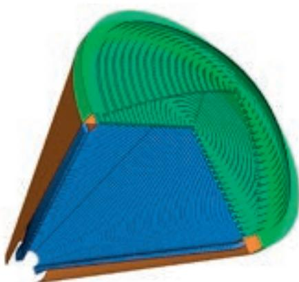
The capability of handling dielectric material in the moment method implementation enables full design and analysis of horn-fed lenses. The picture shows a corrugated horn equipped with a grooved lens.
