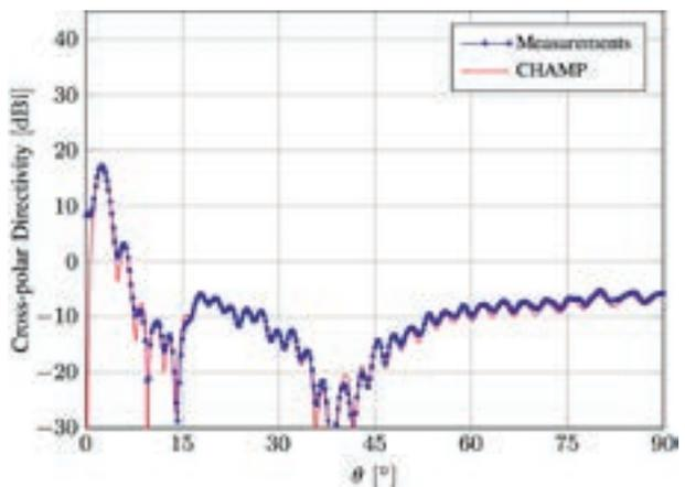
A 44). reflector designed with a dielectrically supported hat-feed and a shaped reflector. All components are optimized by CHAMP, and the measurements carried out at the Technical University of Denmark. A full CHAMP analysis performed in a few seconds reveals the extremely good correlation between measurements (in blue) and predictions (in red).
